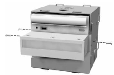
**4.** Slide the device out from the front of the system unit.
